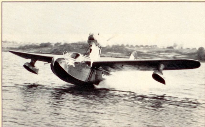
For water landings, the lower struts, which were connected to the fuselage by a solid fairing, lay flat against the hull. The struts were drawn into the hull by an automobile starter motor.
